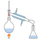
Distillation – separating liquids from liquids based on different boiling points. This can be simple distillation (ink and water) or fractional distillation (crude oil)
